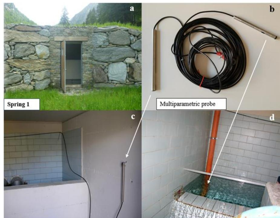
**Figure 3.** Mascognaz 1 spring's structure and set up: (a) External view of the spring water intake structure; (b) Multiparametric probe geometry; (c) Installation of probe data logger; (d) Installation of recording probe.
