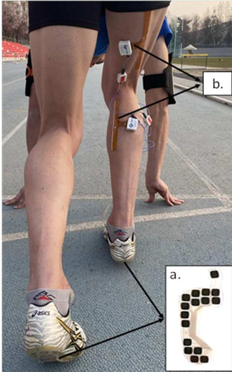
Fig. 1 Subject at the starting position, showing the systems used for the acquisition of kinematics data (a; sensoried insole) and of HD-EMGs (b).
