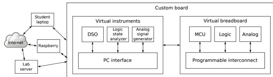
**Figure 1.** Basic architecture of the system.
