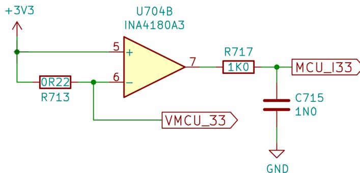
Figure 5. Schematic of a DSO supply current input channel.
