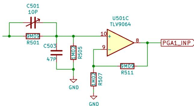
Figure 3. Schematic of a DSO voltage input channel.
