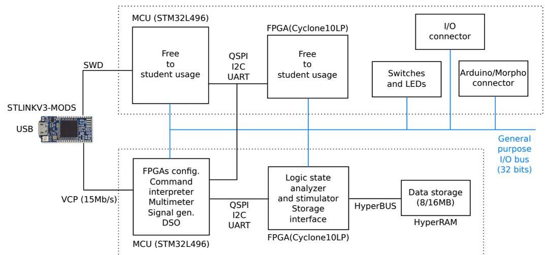
**Figure 2.** Block diagram of the designed board.
