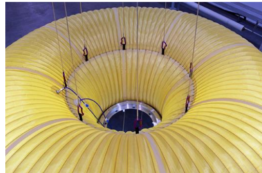
Figure 8: Aft view of the deployed DB-1 HIAD Demonstrator.
