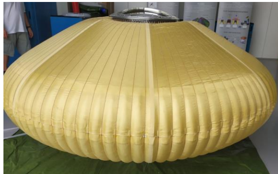
Figure 10: IS static inflation phase (prior to deflection).
