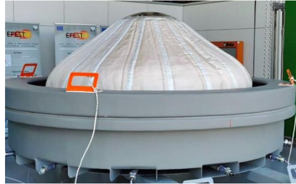
Figure 11 : IAD with integrated F-TPS positioned in static deflection test pool.
