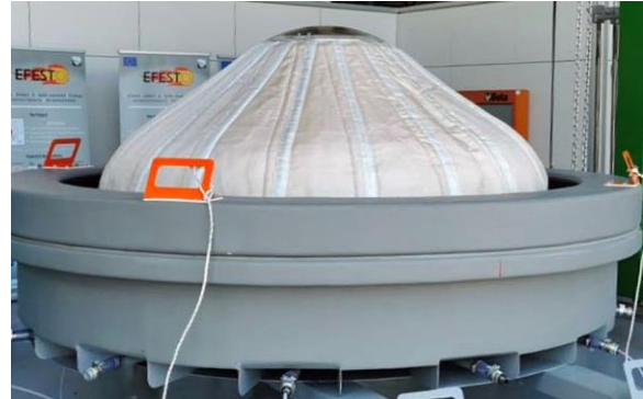
Figure 11 : IAD with integrated F-TPS positioned in static deflection test pool.
