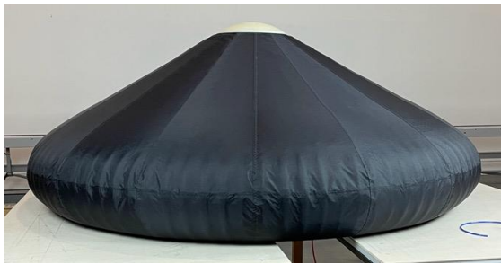
Figure 15: Dual Body EDU incorporating permanent conic profile architecture.
