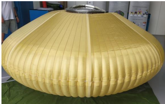
Figure 10: IS static inflation phase (prior to deflection).
