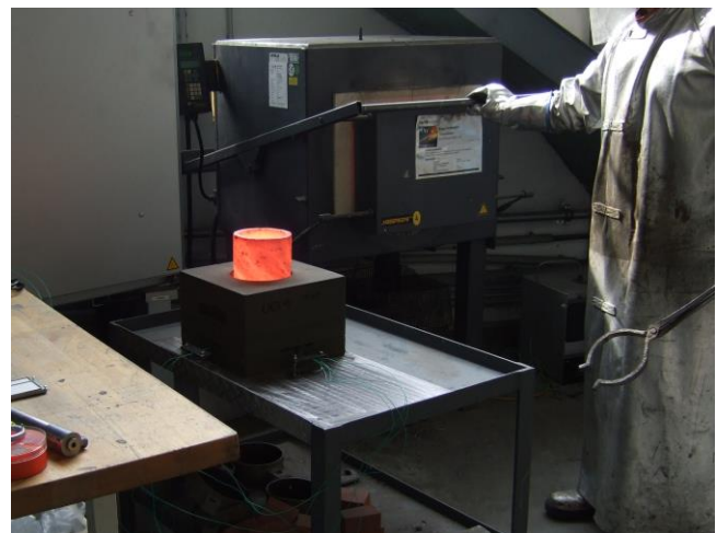
Figure 3: FTPS sample being integrated (left) and the finished sample during the thermal test (right).
