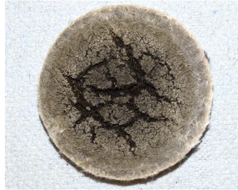
Figure 9: Pyrogel XTE after exposure to 1000°C.
