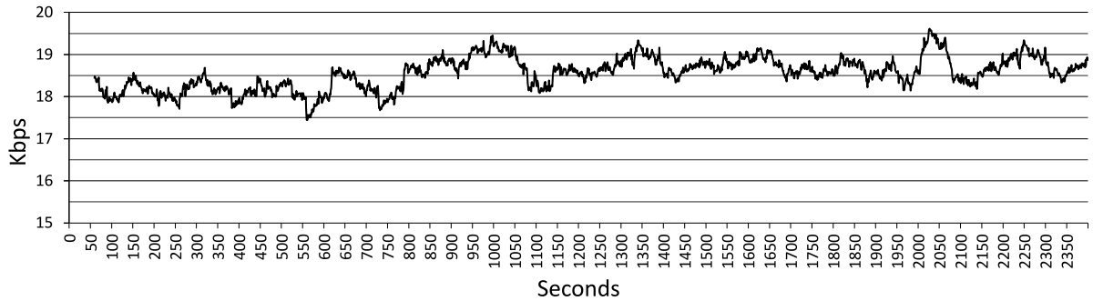
(c) Message bandwidth for the entire ZMQ network layer traffic (CR-RU), excluding the depth data streaming ( \mu = 18.55Kbps , \sigma = 3.20Kbps ).
