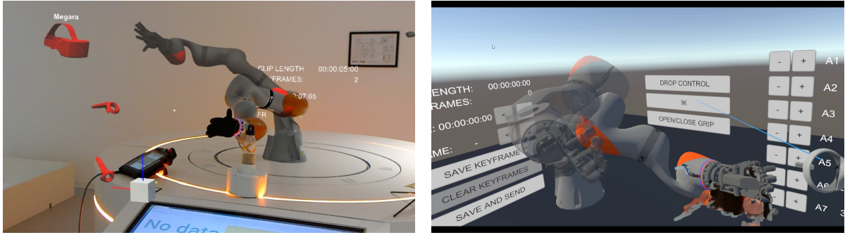
(d) LU's viewpoint while spectating the virtual replica of the RU that interacts with the virtual CR (superimposed on the real one). (e) RU's viewpoint while observing the DT of the (real) CR, the virtual CR, and the point cloud of the workpiece and interacting with the VR UI to create a new program clip.
