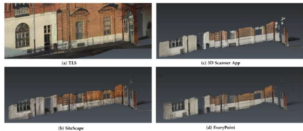
Figure 15. Point clouds derived from the different acquisitions performed on Case Study C.
