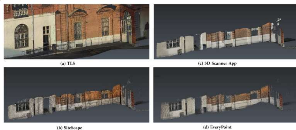
Figure 15. Point clouds derived from the different acquisitions performed on Case Study C.
