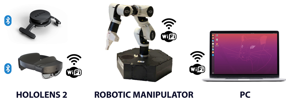
Figure 2. Hardware architecture of the proposed solution.
