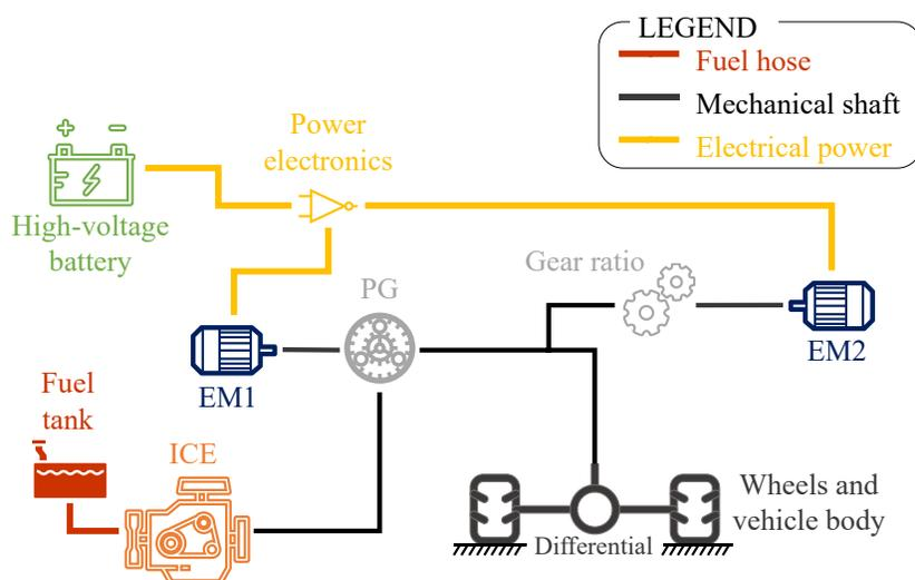
Fig. 1 Toyota Prius hybrid electric powertrain scheme.
