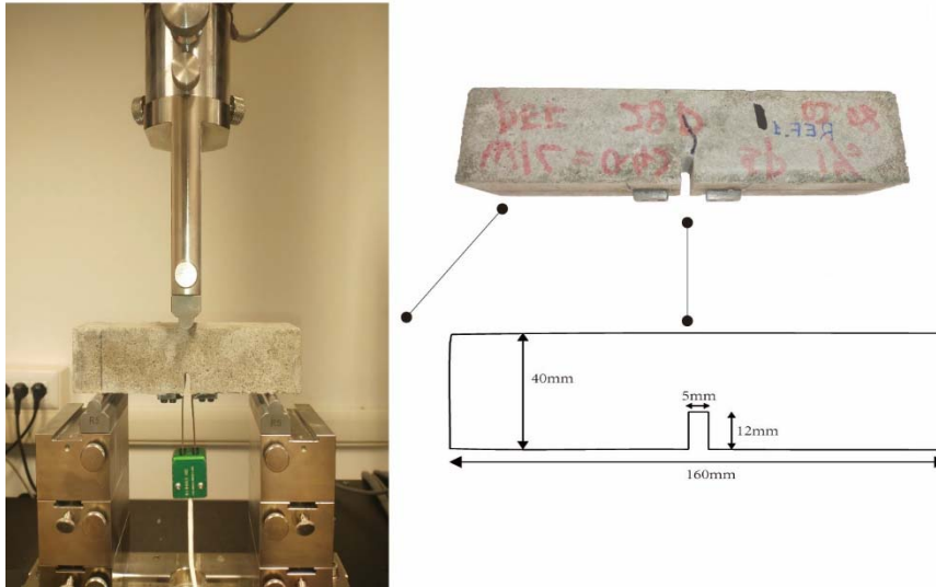
Fig.2. The apparatus for flexural tests
