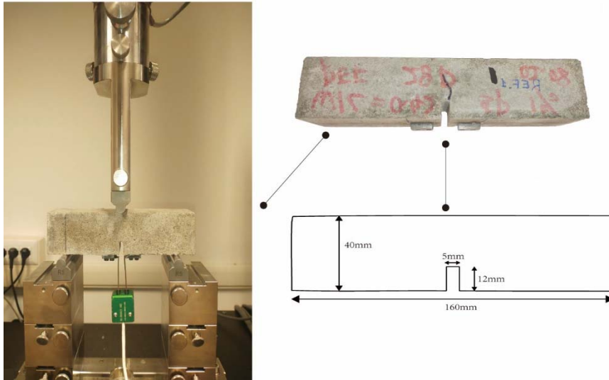
Fig.2. The apparatus for flexural tests
