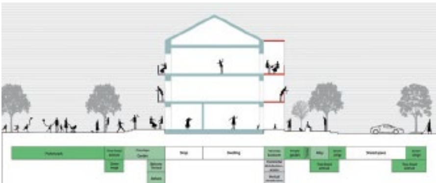
Fig. 4 Cross section of the refurbishment for the Fresia Buildings: continuity between private, semi-private or semi-public, and public space
