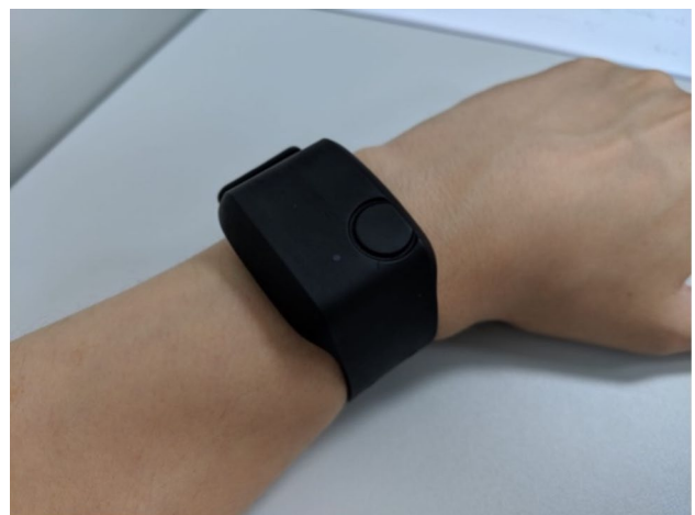
Fig. 3 The Empatica E4 biosensor used for the experiment [35]
