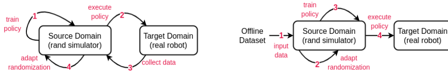
Fig. 1: Conceptual illustration of online (left) and offline (right) adaptive domain randomization.
