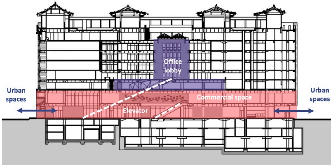
Figure 2.3 Renewal of building-urban interface in Longfu Building
