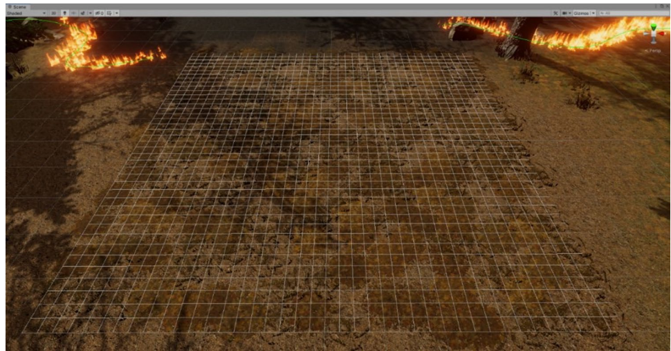
Fig. 5 Visualization of the Terrain Grid when the size of a single tile is set to 25 cm×25 cm. The grid is superimposed to the terrain, where foliage and grass/shrubs have been spawned
