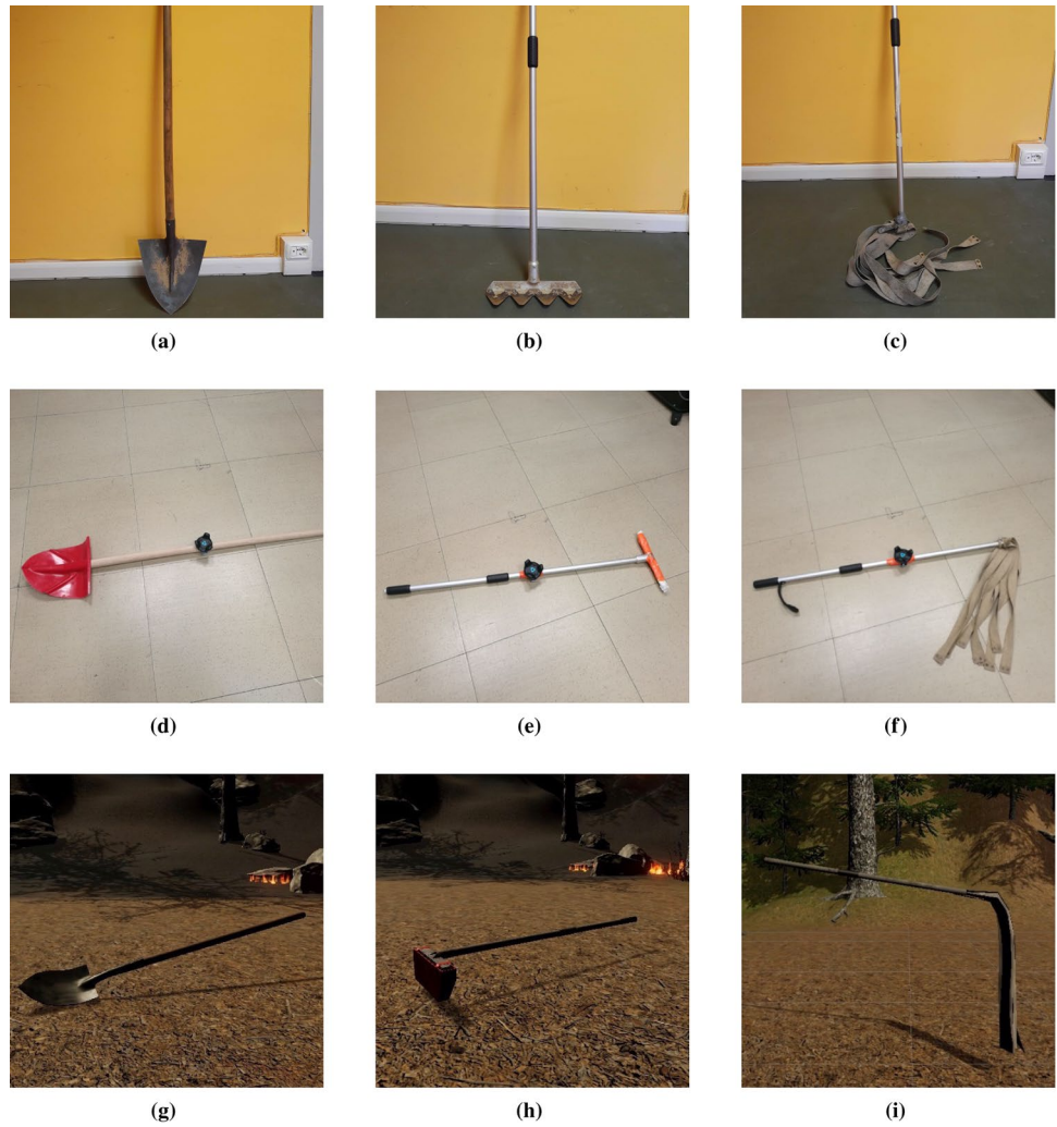
Fig. 3 Firefighting tools: shovel, rake, and beater. Real tools (a–c), Passive haptic interfaces (d–f), and 3D models used in the VR experience (g–i)
