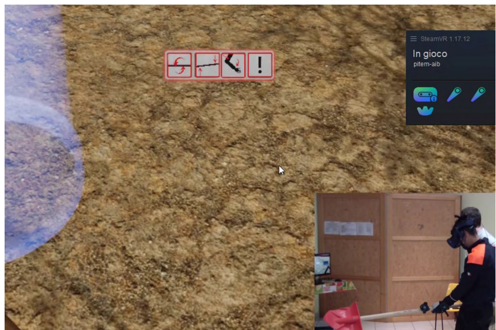
Fig. 9 Guided Mode, transportation phase, performative part; the trainee is asked to grab the shovel and follow a moving target in the scene. The icons show four errors (from left to right): the blade of shovel is not oriented outward, the shovel is not grabbed at the balance point, the trainee's posture is not correct, and a danger situation is found since, in the particular case, the blade of the shovel is out of the trainee's field of view
