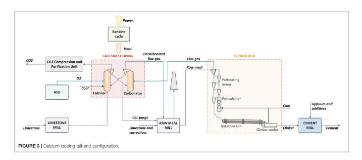
efficiency from the flue gas ( $E_{carb}$ ) of 90%.  $E_{carb}$  can be obtained from the reactor mass balance as a function of the molar flows of CO<sub>2</sub> ( $F_{CO2}$ ) and CaO ( $F_R$ ) entering the carbonator.
