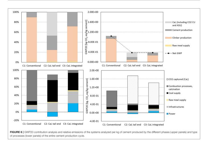
around 1–2% of the overall  $CO_2$ eq emissions. This is more pronounced for GWP20 because of the additional fossil fuel combustion and the associated CH<sub>4</sub> emissions. The addition of CaL reduces the net GWP100 by 68 and 76% and the net GWP20 by 60 and 71% for C2 and C3, respectively, with respect to the reference case, with the CaL-integrated configuration thus exhibiting a substantially improved potential for decarbonization of the cement production cycle.
