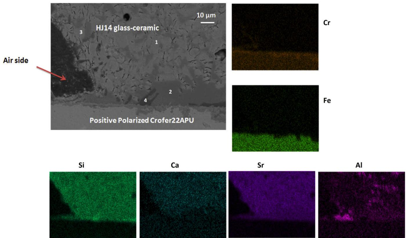
**Figure 6.** SEM image and EDS mapping of the air side of the positively polarized Crofer22APU/HJ14 glass-ceramic interface.
