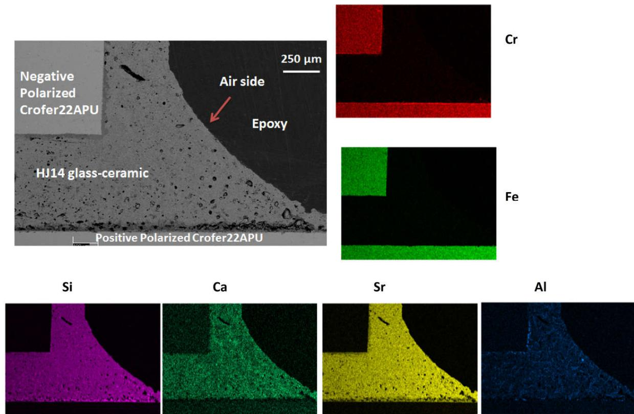
**Figure 5.** SEM post-mortem analyses of the air side of the Crofer22APU/HJ14 glass-ceramic/Crofer22APU joined samples after a thermal aging of 1000 h at 850 °C under an applied voltage of 1.6V.
