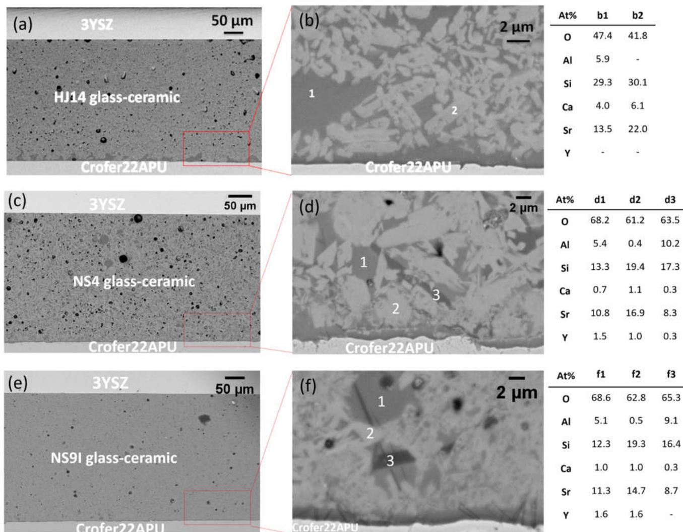
**Figure 3.** SEM backscattered electron images of the as-joined Crofer22APU/glass-ceramic/3YSZ joined samples at different magnifications, together with an EDS elemental analysis (at.%) of the marked points: HJ14 glass-ceramic (a,b); NS4 glass-ceramic (c,d); NS9I glass-ceramic (e,f).
