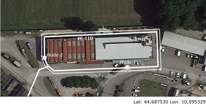
Fig. 3: Top view of the test site with schematic representation of the water pipe and location of the nodes. The length of the two main propagation paths is highlighted. The designation PE110 is used for the identification of the pipe properties.
