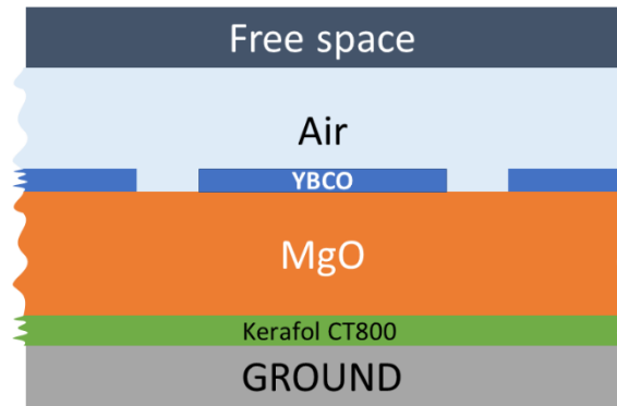
Figure 50: Schematic view of the layers in SONNET®
