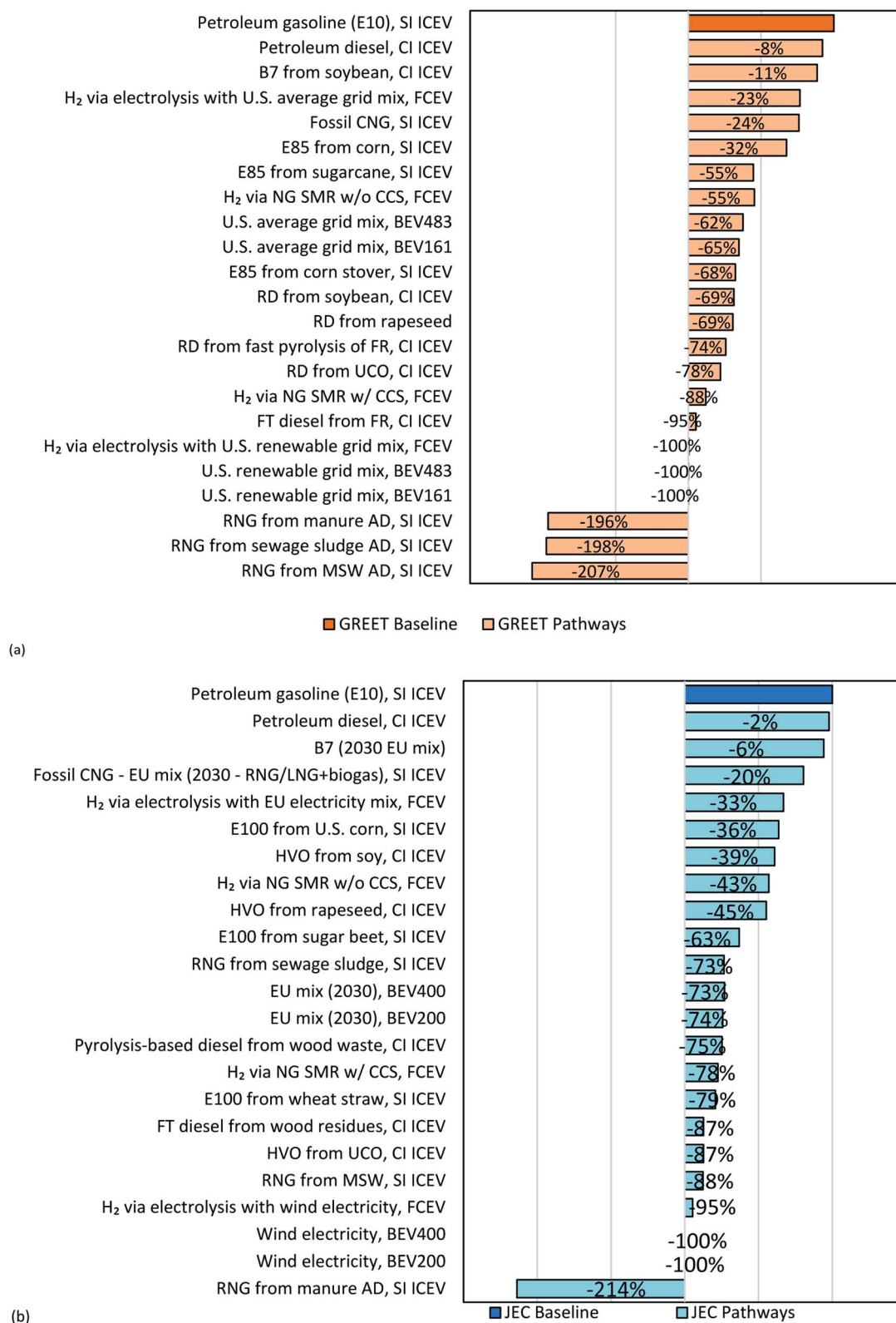
Fig. 4 Per km WTW GHG emission reductions of fuel-vehicle technologies compared with baseline gasoline (E10) ICEV (a) in the United States according to GREET and (b) in the EU according to JEC v5. The results are normalized to the U.S. petroleum gasoline vehicles and EU petroleum gasoline vehicles as the baseline, respectively.
