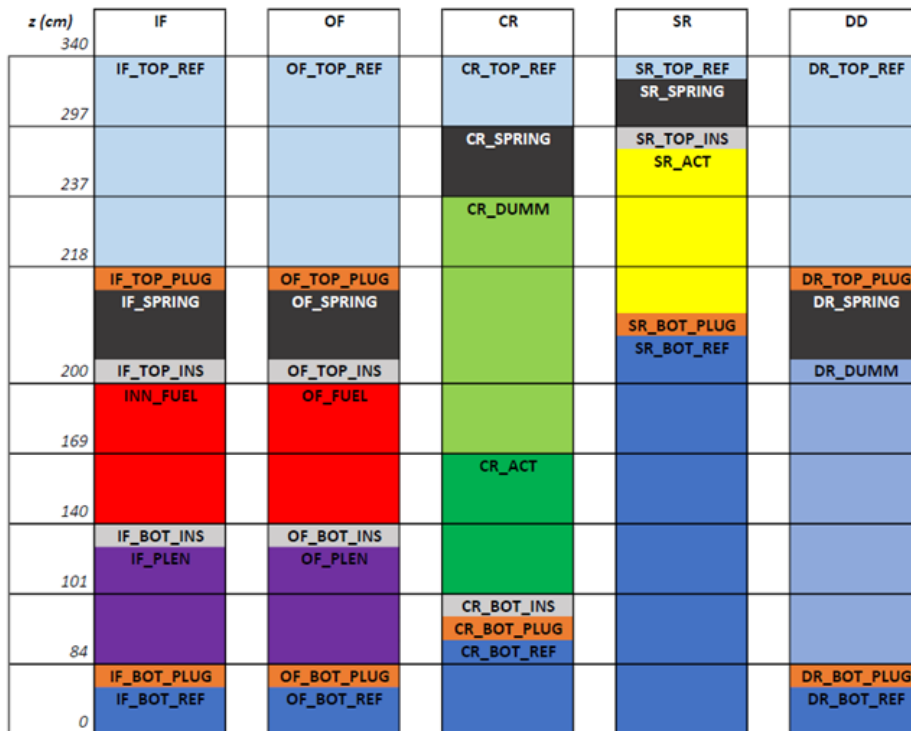
Figure 2.18: ALFRED core configuration with CRs position adjusted to reach a condition closer to criticality.
