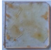
Figure 129: Few red aggregates on the glass that probably indicate a surface crystallization
