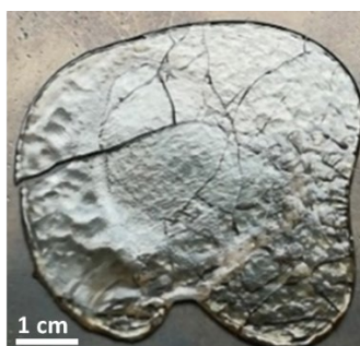
Figure 8: Example of LNS glass plate after the glass cooling (typ. 5cm size and few mm thick)
