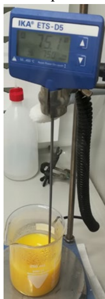
Figure 126: Solution of first attempt with a probe to maintain a constant temperature of 75°C during the process
