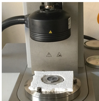
Figure 3.5 DSR conditioning hood for MTL test
