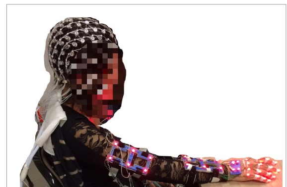
Figure 2. Exemplary experimental setup. High-resolution EEG sensors and active optical markers are mounted on the subject for motion tracking.
