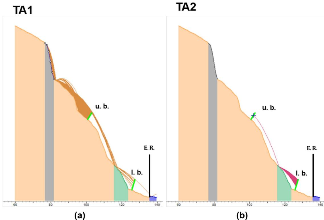
**Fig. 5** Trajectory analyses on the considered path (RocFall v 8.017). See Table 1 for details on input parameters: simulations TA1 (a) and TA2 (b) with a 8 m height net fences. The element at risk (E.R.), i.e.
