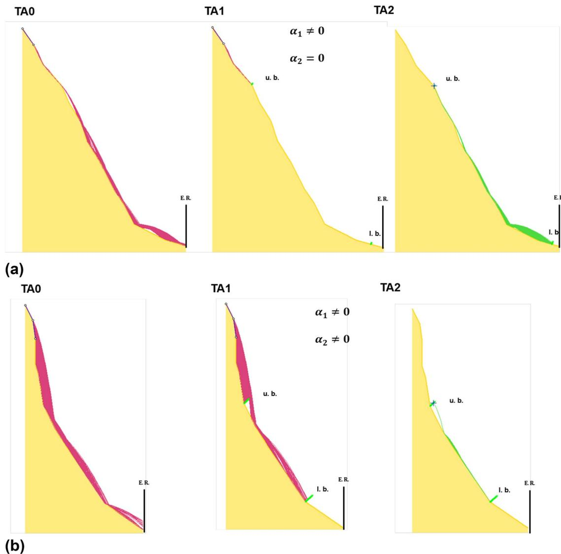
**Fig. 3** Visual flowchart of the proposed rigorous method for the design of the double line system: in case of **a** a full or **b** partially interception of blocks by the upslope net fence. In both cases,  $\alpha_1 \neq 0$ , i.e. not all the intercepted blocks are stopped by the upper line. The
