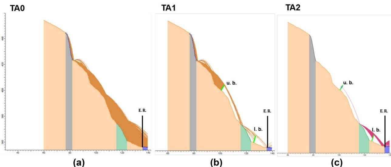
**Fig. 4** Trajectory analyses on the considered path (RocFall v 8.017). See Table 1 for details on input parameters: **a** simulation TA0 without any barrier **(a)**, simulations TA1 **(b)** and TA2 **(c)** with the selected barriers. The element at risk (E.R.), i.e. the infrastructure, is indicated
