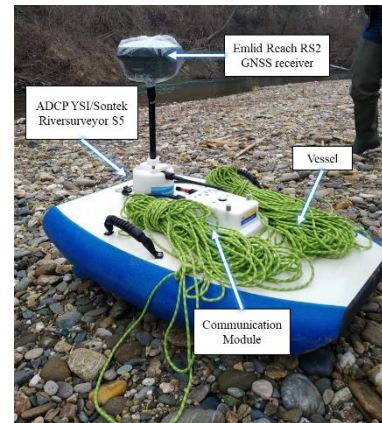
Figure 6. ADCP mounted on the mobile vessel.
