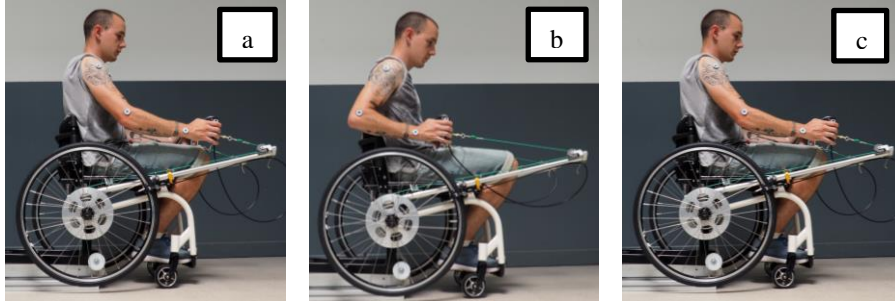
Figure 5: Innovative system of propulsion applied on a standard wheelchair.
