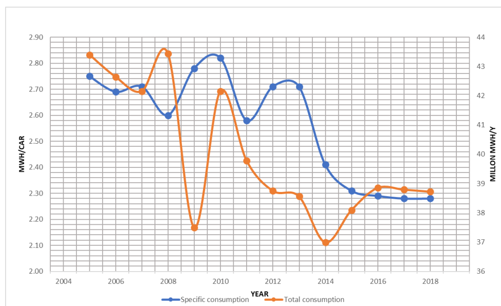
Figure 1. Energy consumption during car production in automotive industry (source: ACEA, 2019 [20]).
