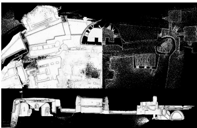
Figure 4. SLAM Point Cloud of the interior and exterior of the bastion of Qal'at al-Bahrain. Source: authors and BACA.
