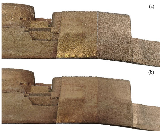
Figure 15. LiDAR point optimisation (filtering and radiometric balancing). (a) LiDAR point cloud before the optimisation; (b) LiDAR point cloud after the optimisation.
