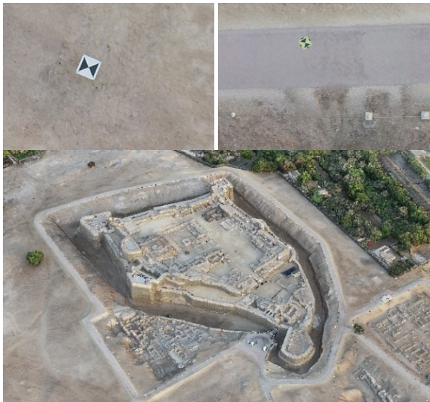
Figure 3. UAV Dense Cloud of Qal'at al-Bahrain, flight altitude 100m. Source: authors and BACA.
