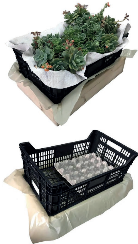
Figure 22 | The constructed Blue-Green Roof Module prototype. Source: Caterina Dadati and Marco D’Amico.
