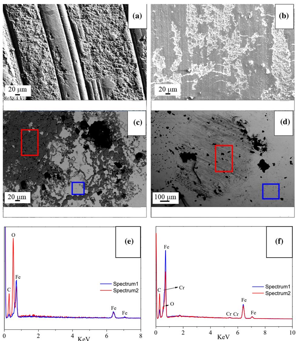
severe wear losses, whereas the worn surface of EP/HFB 90/10 composite (reported as example for the composites in Fig. 9B) is much smoother and the signs of adhesion, deformation and exfoliation of
