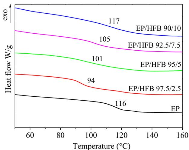
**Figure 6** DSC traces of epoxy-hemp fiber biochar composites.
