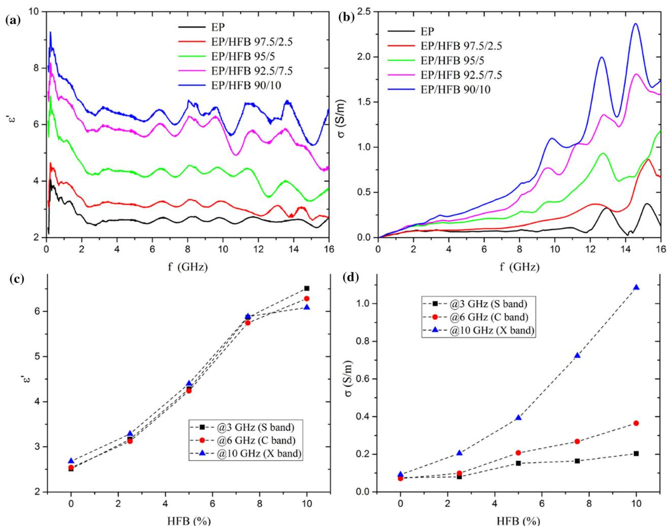
**Figure 11** Real part of the complex permittivity **a** and conductivity **b** as a function of frequency, and complex permittivity **c** and conductivity **d** as a function of HFB weight fraction at representative frequencies for communication microwave bands.
