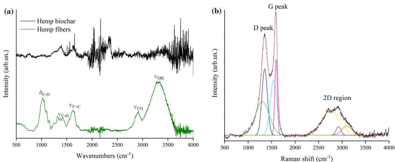
**Figure 2** (a) FTIR spectra (ATR mode) of pristine (green) and pyrolyzed (black) hemp fibers and (b) Raman spectra HFB in the range from 500 to 4000  $\text{cm}^{-1}$ .
