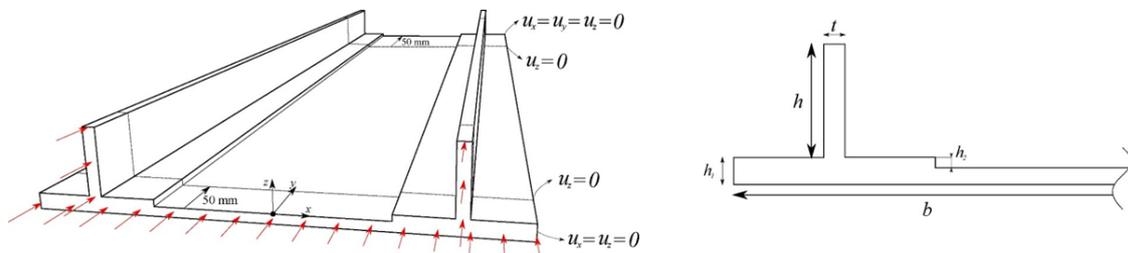
Figure 1. Panel dimensions (left) and stiffener dimensions (right)
