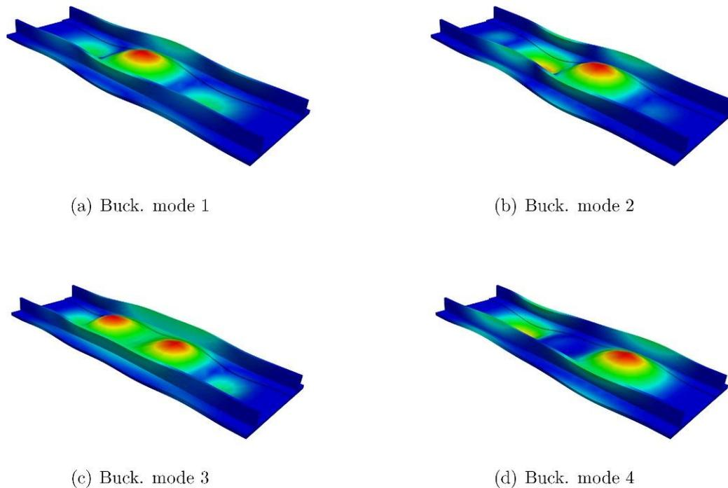
Figure 2. buckling modes from finite element simulations
