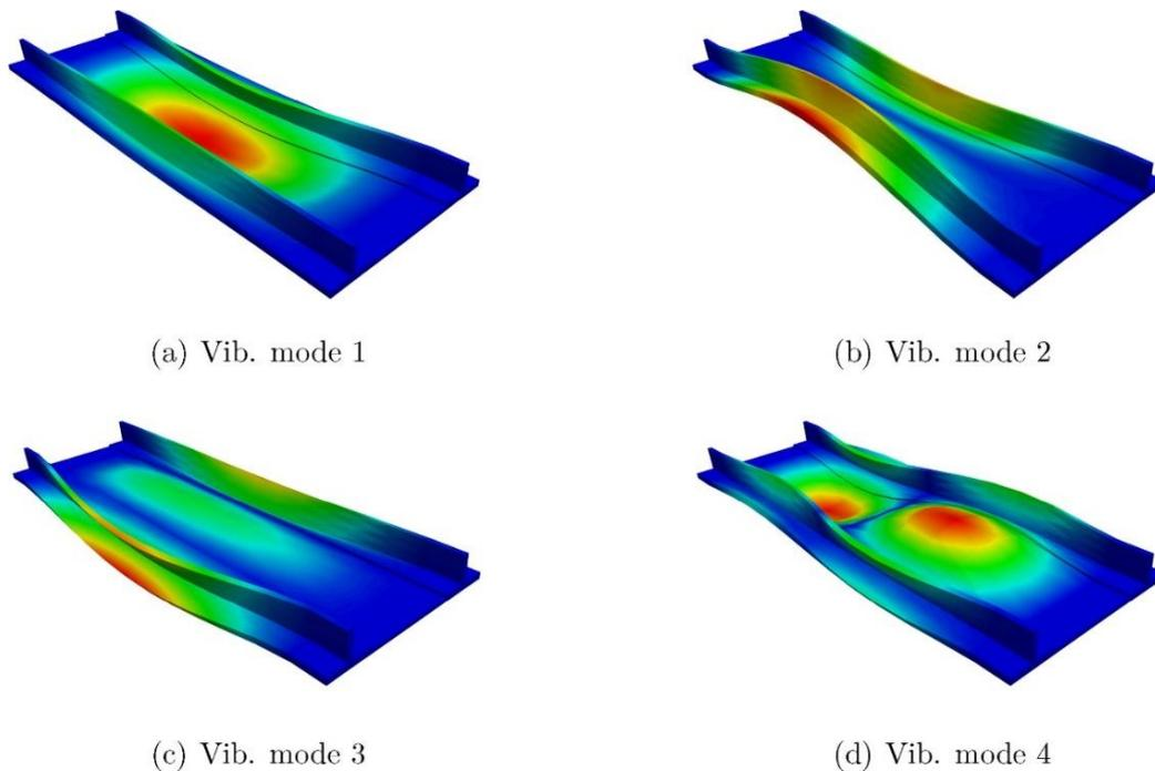
Figure 7. vibrations modes obtained from CUF model
