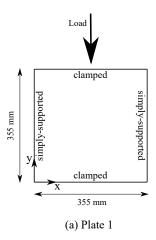
**FIGURE 1**: GEOMETRY AND BOUNDARY CONDITIONS OF THE ALUMINIUM FLAT PLATE.
