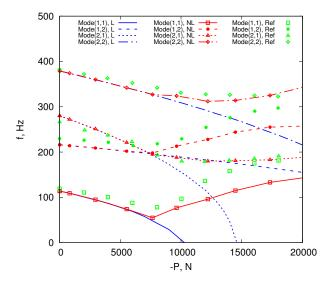
**FIGURE 5**: COMPARISON BETWEEN LINEAR, NONLIN-EAR AND EXPERIMENTAL VARIATION OF THE NATU-RAL FREQUENCIES OF THE ALUMINIUM FLAT PLATE FOR PROGRESSIVELY INCREASING LOADINGS.
