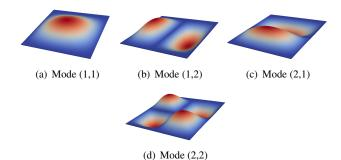
**FIGURE 4**: CHARACTERISTICS FIRST FOUR VIBRATION MODE SHAPES FOR THE ALUMINIUM FLAT PLATE. *P*= 0 N.
