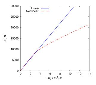
**FIGURE 2**: LINEAR AND NONLINEAR LOAD-DEFLECTION CURVE. ALUMINIUM FLAT PLATE SUB-JECTED TO COMPRESSIVE LOAD.
