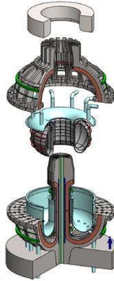
**Figure 1: ARC assembling scheme (reproduced from [1]).**
