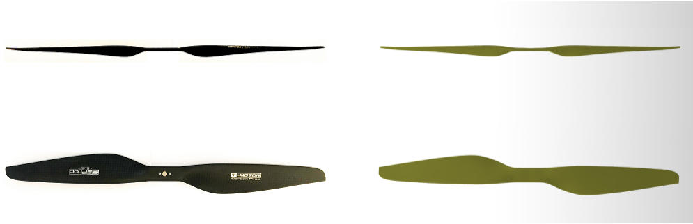
Fig. 3 Comparison of top and front views of the original (left) and digitally reconstructed (right) blade.
