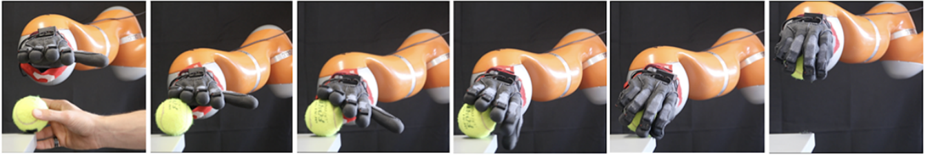
Fig. 7: Snapshots of one experiment performed on a table. Contact was on the L/R zone with the hand following traj. 1.
