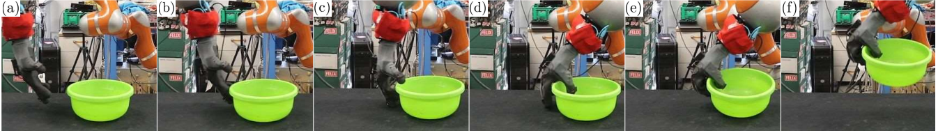
Fig. 8. Photosequence of a grasp produced by the proposed architecture during validation: Bottom grasp of object 14. The hand starts from the initial configuration of the primitive in panel (a). The contact happens in panel (b), triggering the reactive routine. In panel (f) the object is firmly lifted.
