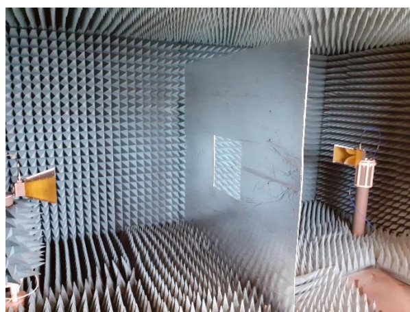
Figure 5. Measurement setup for transmission measurements of the drywall.
