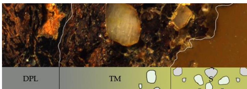
Figure 5. The schematic corrosion layers correlated with the section of sample CH_03. The soil layer (S) is not present anymore, because the sample was cleaned before the inclusion in resin.
