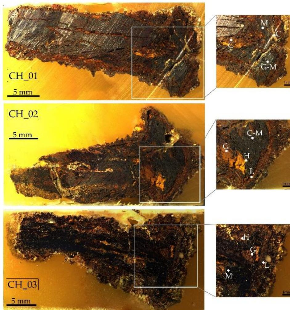
**Figure 6.** Cross-sections of the nails from Tharros with the identification of the different corrosion products by Raman spectroscopy. G = goethite, M = magnetite, H= hematite, L = lepidocrocite, G-M = mixture of goethite and magnetite.
