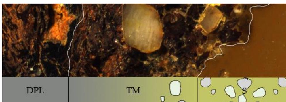
**Figure 5.** The schematic corrosion layers correlated with the section of sample CH\_03. The soil layer (S) is not present anymore, because the sample was cleaned before the inclusion in resin.
