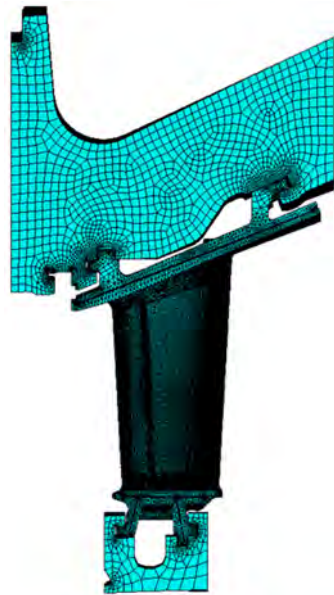
Figure 2. Finite element (FE) model of a turbine vane with its turbine vane carrier (TVC) and U-ring sector.
