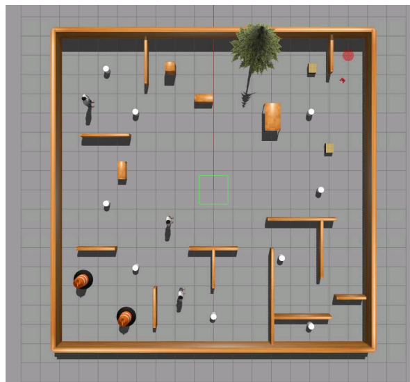
Fig. 1. Representation of a common simulated environment for training an agent. If robot dynamics and task constraints are correctly encapsulated into the simulation, it is possible to deploy on the real setting with minimal loss of performance.
