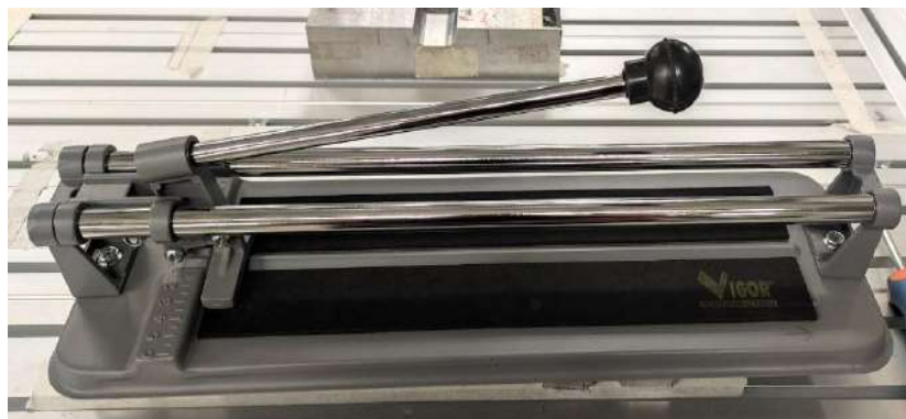
Figure 2 - Final assembly of the tile cutter (44 x 14 x 9 cm).
