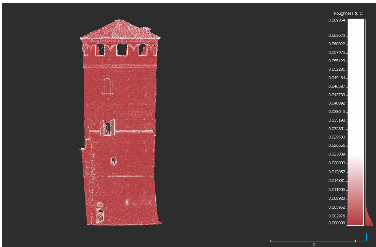
Figure 28. Roughness analysis of the photogrammetric data: RMSe 0.006 m; standard deviation 0.005 m. White points are related to roughness and noise record.
