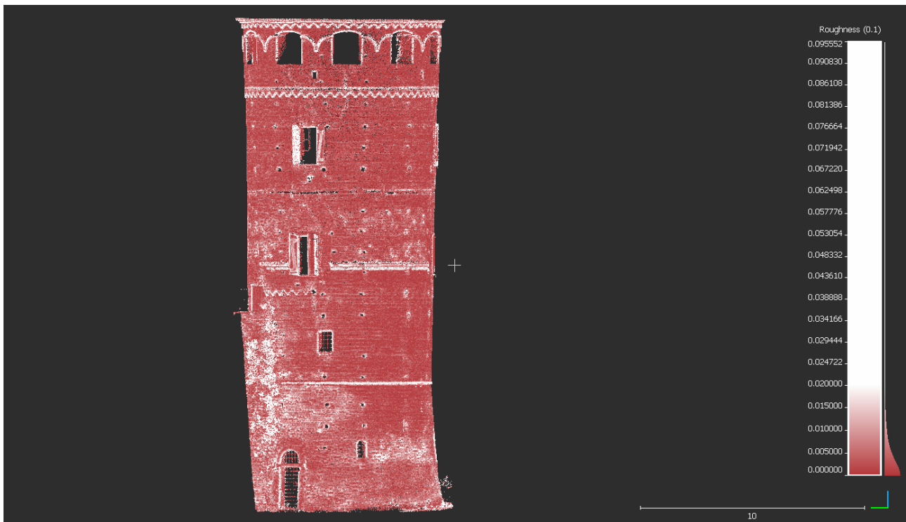
Figure 27. Roughness analysis of Trimble SX10 data: RMSe 0.009 m; standard deviation 0.007 m. White points are related to roughness and noise record.
