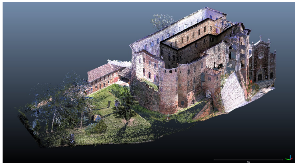
Figure 4. Trimble SX10 external point clouds of the castle and surroundings (point dimension 1 pixel).
