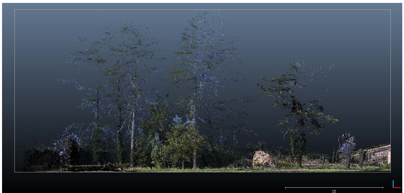
Figure 34. Vegetation of the castle captured by the Trimble SX10 scanning station.
