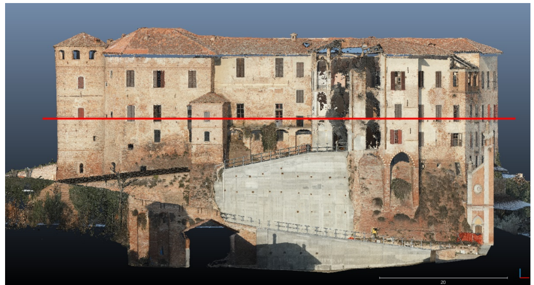
Figure 17. Profile 3 on the z axis, slicing only the castle at 11.50 m from the terrain level.
