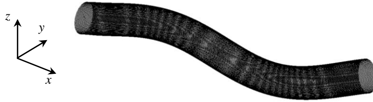
Figure 12: 3 rd flexural mode (3F, f = 1,835 Hz).
