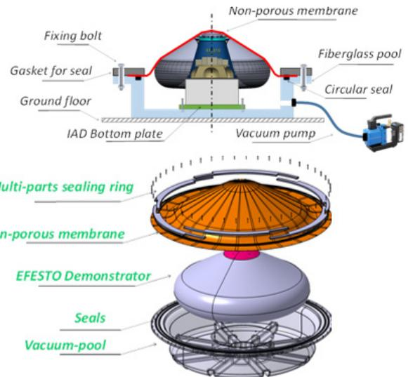
Figure 32 EFESTO Ground demonstrator– Static Load test.
