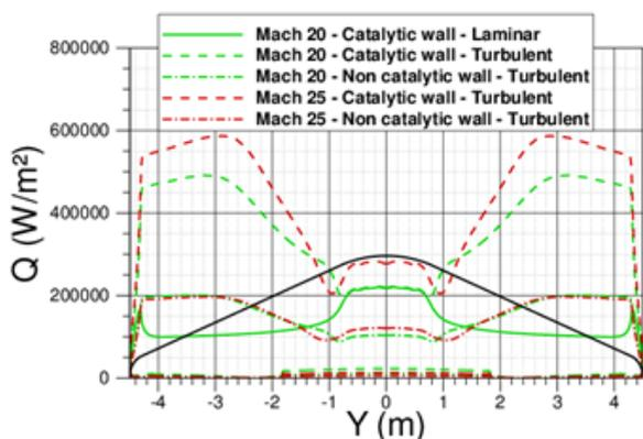
**Figure 10** Influence of catalycity and laminar/turbulent boundary layer on the wall heat flux for the flight points [35 km, Mach 25] and [24 km, Mach 20] - CFD CEDRE simulations - Mars mission.
