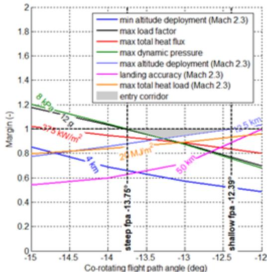
**Figure 14** Mars, entry corridor. Variability of trajectory margins with respect to constraints as a function of the flight path angle at the EIP.
