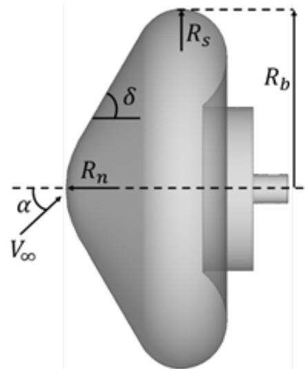
Figure 8 Geometrical parameters.
