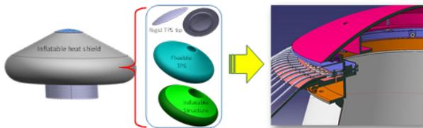
Figure 29 EFESTO 1:2 Ground Demonstrator – CAD model.
