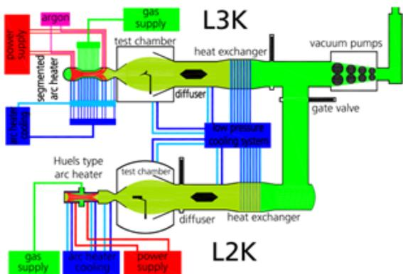
Figure 26 DLR's arc-heated facilities LBK.
