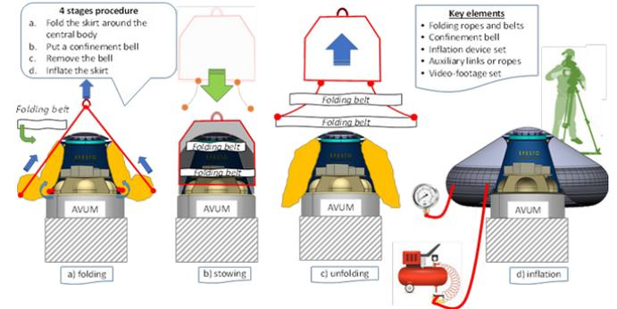
Figure 31 EFESTO Ground demonstrator – Inflation and Deployment test.
