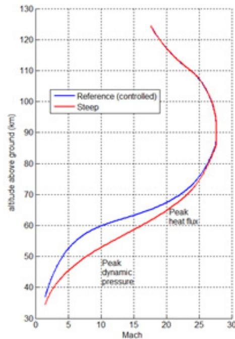
Figure 13 AVUM, sizing and reference (controlled) entry trajectories.
