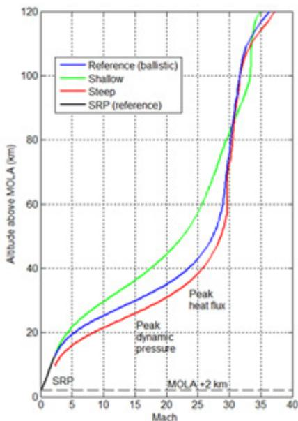
**Figure 15** Mars, sizing and reference (ballistic) trajectories.
