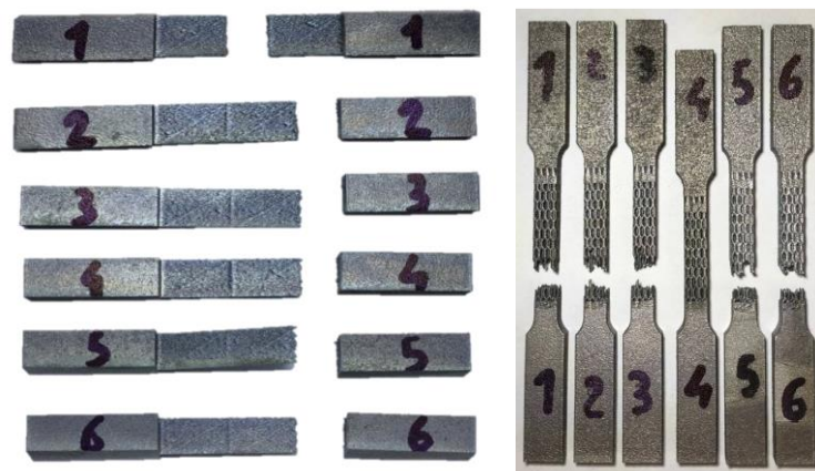
Fig. 1. Samples for tensile characterization of bulk and lattice supports.
