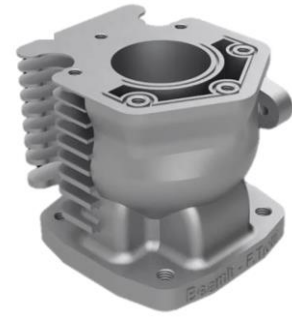
(a) (b) Fig. 2. Target cube objet with significant features (a) and engine cylinder component (b) used for the optimization and validation of the sandblasting-driven supports release.
