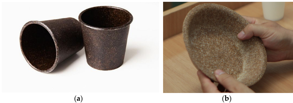
Figure 6. Biodegradable disposable tableware: (a) a laboratory prototype of disposable tableware based on biomaterial from spent coffee grounds ( Open source photo ) [50]; (b) biodegradable disposable tableware based on the meal ( Open source photo ) [58].
