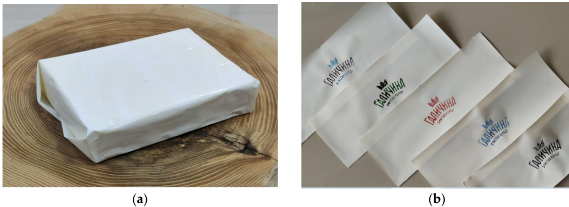
Figure 5. (a) Biodegradable eggshell packaging for food; (b) biodegradable eggshell labels for bottles ( Open source photo ) [57].
