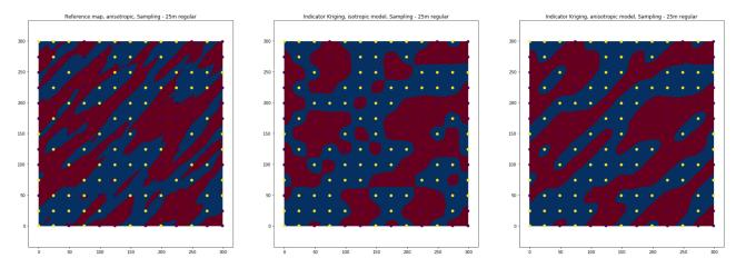
Figure 5 – Comparing the results from isotropic IK and anisotropic IK with the reference map.
