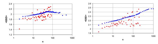
Figure 3 – Dependence of the mean empirical GSD,  $\langle GSD \rangle$ , within cells on sample size (n) per cell. Left: German dataset, Right: European dataset. Red: Mean GSD of cells with n measurements; blue: mean GSD of cells with  $\geq$  n measurements.
