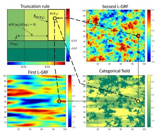
Figure 1 – Example of a pluriGaussian simulation with two uncorrelated L-GRFs. The dotted arrows represent an example of truncation described by Eq. 2. An example of notions of facies domain  $(\mathcal{D}(T_j))$ , facies boundary  $(S_{\mathcal{D}(T_j)})$  and distance  $(d_k(Y(x_k)|\mathcal{C}(x_k)=j))$  is shown on the truncation rule for the yellow facies (facies 5) (See Eq.3 and Eq.4).
