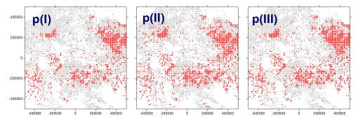
Figure 6 – Radon priority areas (red) in Central Europe, defined as prob(Rn>300 Bq/m³)≥0.1, calculated with 3 different models. Blank: cells with less than 2 measurements.
