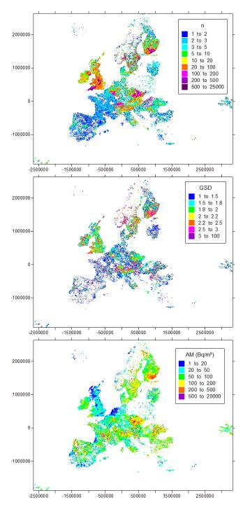
Figure 4a – European indoor Rn dataset (version 2019): n – number of observations per cell; GSD – geometrical standard deviation, AM – arithmetical mean Rn concentration per 10km×10km cell.
