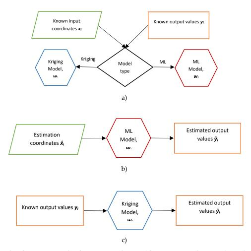
Figure 1 – Machine learning approach vs kriging approach: a) model construction to obtain weights w<sub>i</sub>; b) estimation with ML algorithm; c) estimation with kriging algorithm.
