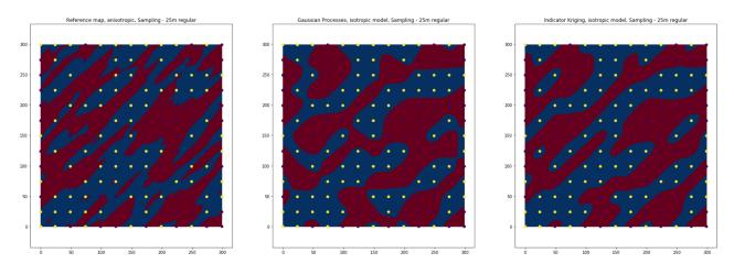
Figure 6 – Comparing the results from Gaussian Processes and anisotropic IK with the reference map.
