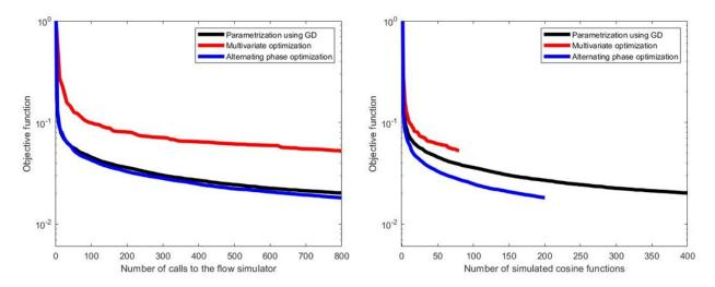
Figure 4 – Comparison of three optimization strategies. Left) based on the number of calls to the flow simulator. Right) based on the numbers of simulated cosine functions. (Black: parametrization using gradual deformation; Red: multivariate optimization using a Nelder–Mead method; Blue: univariate optimization using an alternating scheme with one phase at a time).
