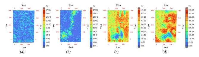
Figure 4 – Conditional variance maps of Al2O3 for (a) TBSIM and (b) TBCOSIM and of Fe for (c) TBSIM and (d) TBCOSIM obtained from (alr) transformation.
